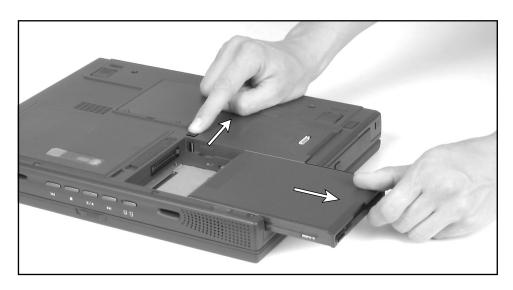
**3** Firmly push the second battery straight into the bay until the latch clicks into place.
