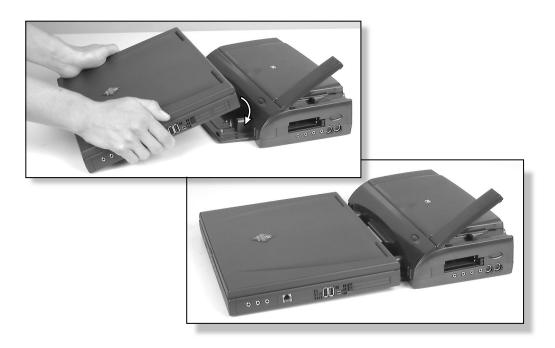
**5** Press down on the release latch until it snaps into place.
