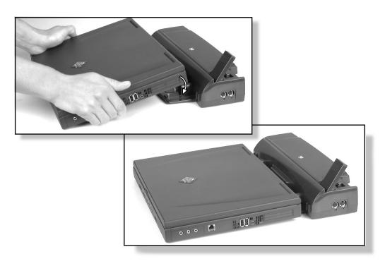
4 Press down on the release latch until it snaps into place.
