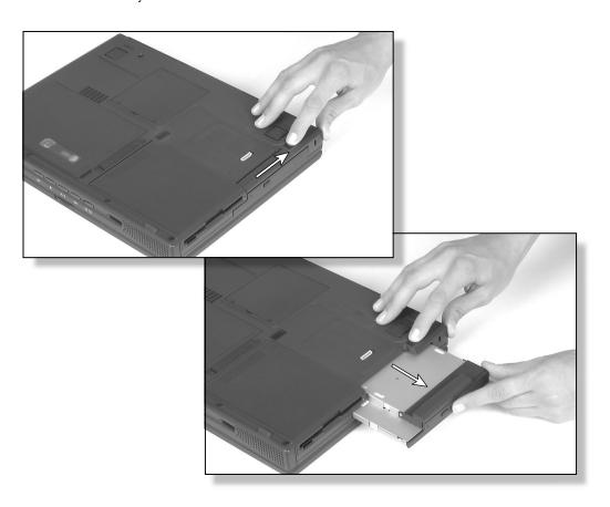
Firmly push the new module straight into the bay until the latch clicks into place.
