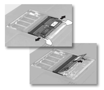
**4** Pull the memory module out of the slot.
