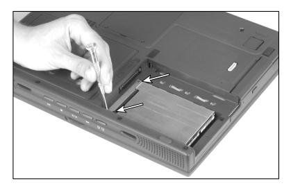
Slide the hard drive away from the connector and remove it from the bay.
